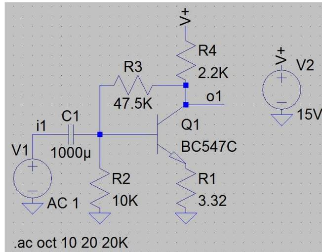
Fig. 1b Example common emitter gain stage
