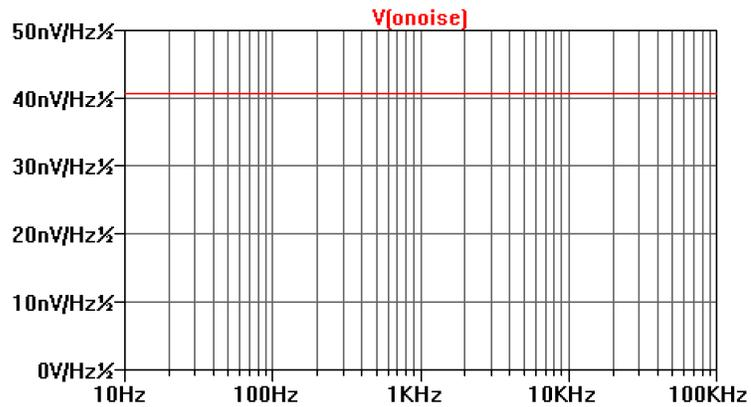
Fig. 7b LTspice created noise voltage density trace from the Fig. 7a output o1
