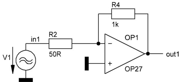
Fig. 1a Test circuit of an OP27 driven amp in inverting configuration
