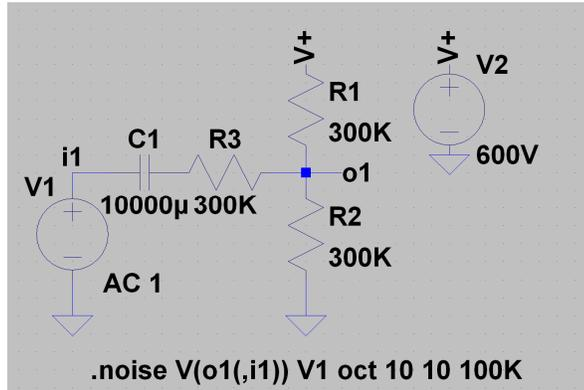
Fig. 7a Test circuit for the evaluation of resistor excess noise
