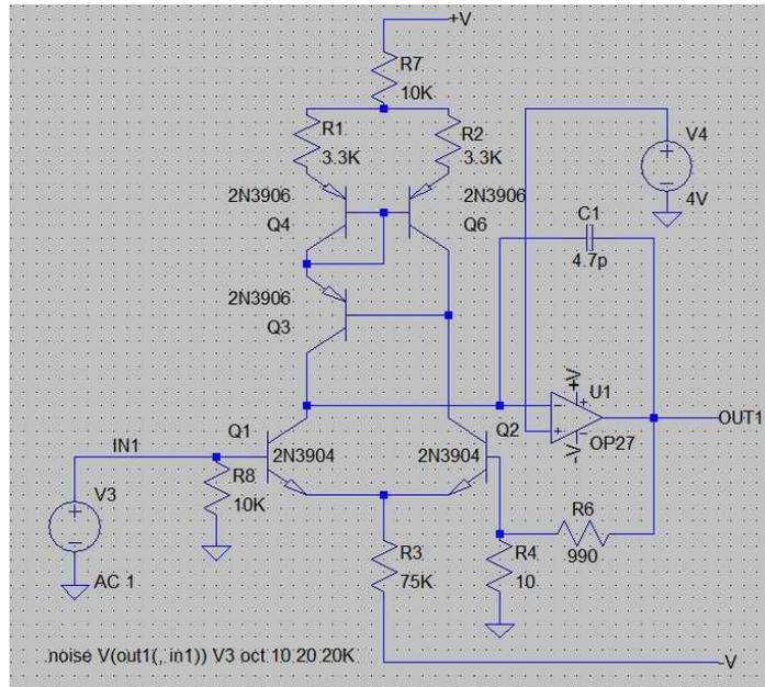
Fig. 3 Non-inverting example amp with a signal gain of 100
