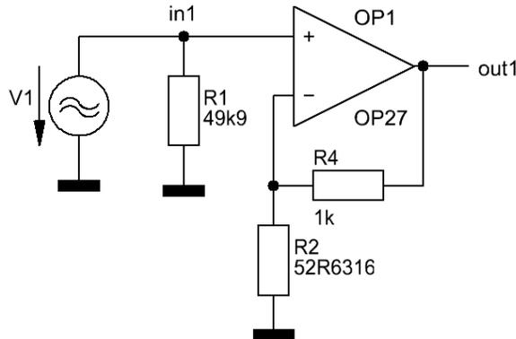
Fig. 2 Test circuit of an OP27 driven amp in non-inverting configuration
