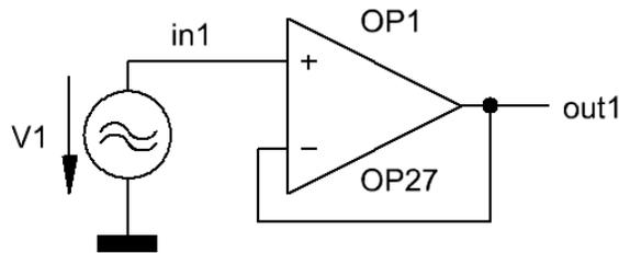
Fig. 5 Test circuit to get the input noise voltage of an op-amp via  $V(\text{onoise})$
