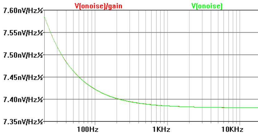
Fig. 4 Input referred noise voltage density trace (red & hidden) and output noise voltage density trace (green) of the Fig. 2 arrangement with a gain of 2
