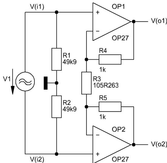
Fig. 6 Balanced amp configuration with a balanced signal gain of 20
